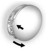
The fuel cap is located behind a hinged fuel door on the passenger side of the vehicle. To open the fuel door, push the rearward center edge in and release and it will open.
