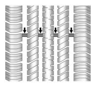
Treadwear indicators are one way to tell when it is time for new tires. Treadwear indicators appear when the tires have only 1.6 mm (1/16 in) or less of tread remaining. See *Tire Inspection on page 10-68* and *Tire Rotation on page 10-68* for more information.
