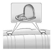
Be sure to use an anchor on the same side of the vehicle as the seating position where the child restraint will be placed. Do not secure a child restraint in a position without a top tether anchor if a national or local law requires that the top tether be attached, or if the instructions that come with the child restraint say that the top tether must be attached.
