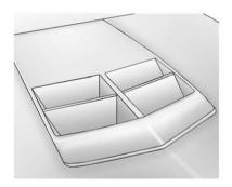
It is not recommended that the air extractor on the ZL1 be waxed, as it will change the gloss level of the surface. In addition, care must be used when waxing around the air extractor. If a small amount of wax is applied to the extractor it can create an irregular appearance in the surface of the panel. If wax, debris, or other materials create stains on the air extractor, see your dealer for the recommended cleaner
