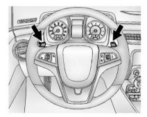
Vehicles with any axle other than GW8 have a Tap Shift Mode. Tap Shift allows the driver to manually control the automatic transmission. To use Tap Shift, the shift lever must be in M (Manual Mode). Vehicles with this feature have indicators on the steering wheel. The controls are on the back of the steering wheel.
