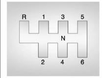
These are the shift patterns for the six-speed manual transmissions.
