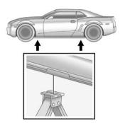
Position the jack lift head at the jack location nearest the flat tire. The location is indicated by a mark on the bottom edge of the vehicle. The jack must not be used in any other position.
