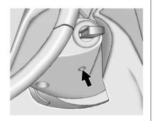
Vehicles with an automatic transmission are equipped with an electronic key lock release system. The key lock release is designed to prevent ignition key removal unless the shift lever is in P (Park).
