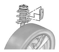
Due to low ramp angles on the ZL1, use care when loading the vehicle onto a flatbed carrier. Front spring spacers are provided for lifting the front suspension.
