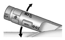
An arrow on the instrument panel cluster flashes in the direction of the turn or lane change.
