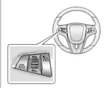
The cruise control buttons are located on the outboard side of the steering wheel.
