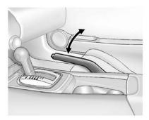
To apply the parking brake, pull up on the parking brake handle. It is not necessary to push in on the release button while applying the parking brake. If the ignition is in the ON/RUN position, the brake system warning light will come on. See Brake System Warning Light on page 5-21.
