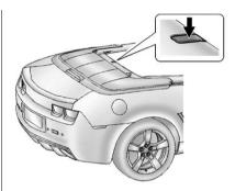
Remove the trim cover to access the hydraulic pressure release bolt.
