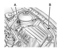
The jump start positive (A) and negative (B) posts are located in the engine compartment on the driver side of the vehicle.
