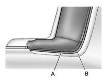
Push the outside rim (A) of the tonneau cover under the vehicle trim (B) on both sides.
