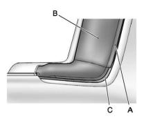
6. Push the edge (A) of the center of the tonneau cover (B) under the vehicle trim (C).
